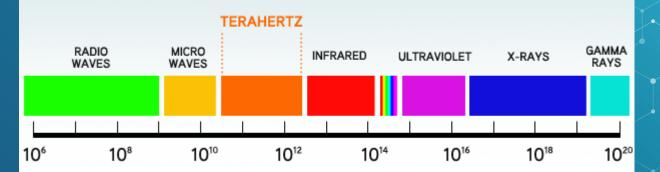
The terahertz spectral region (40GHz to 4THz or 7.5mm to 75µm) sits between microwaves and the far infrared
